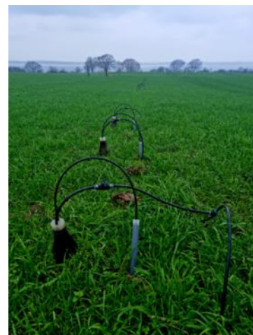
Figure 3. Ceramic suction-cup equipment used to collect soil water for measuring nitrate leaching under pasture conditions.
