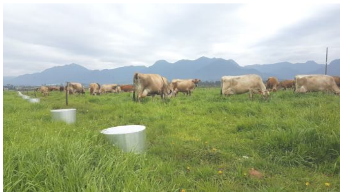
Figure 2. Static chambers used to measure nitrous oxide ( N_2O ) emissions from the soil under field conditions in a pasture-based dairy production system.
