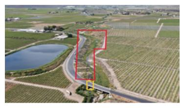
Image 3: Groynes visible inside the red lines, and the historical break in the road next to the bridge indicated inside the yellow lines.
