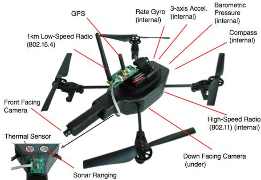
Figure 2: Just some of the sensors deployed on a simple UAV platform Source: http://wise.ece.cmu.edu/redmine/projects/drone-rk/wiki .
