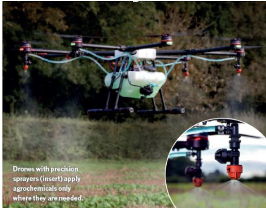
Drones with precision sprayers (insert) apply agrochemicals only where they are needed.
